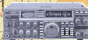
IC 1000 - Potenza 100W RX-TX 100 kHz/30 MHz - Tx: 14, 21, 24, 28 MHz - 100W RF SSB/CW/AM/FM, RTTY
